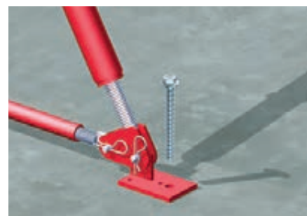
Assembling of supporting props
